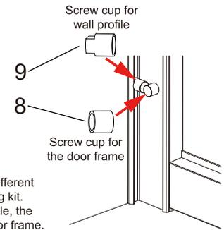
**Note:** There are two different screw cups in the fitting kit. one is for the wall profile, the other one is for the door frame.
